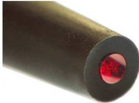
Figure 1.2: Schematic of a plastic optical fibre [140].
