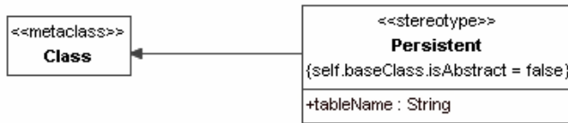
Figure 12.2. An example of a UML 2.0 stereotype specification
